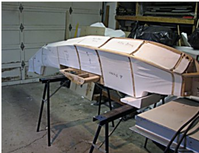
The Stranraer model fuselage, illustrating the method of construction using foam blocks fitted between plywood formers.
