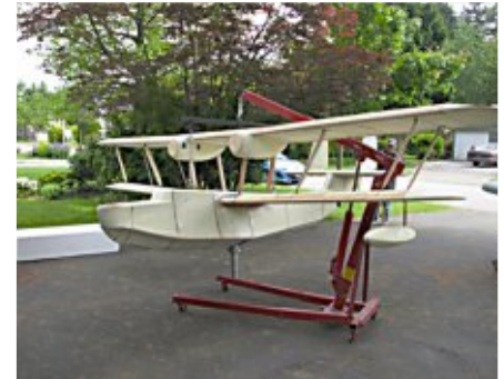
The completed Stranraer hangs from a hoist. Predicting the balance point was a critical challenge, as the model will function as a weather vane, swivelling on its central pole.
